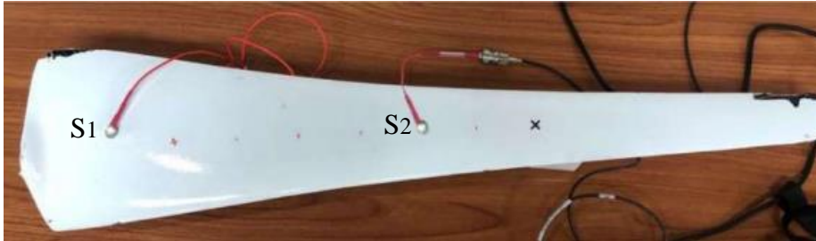
Figure 1. Experimental view of wind turbine blade with two AE sensors.
